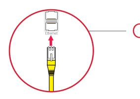
Connect the Ethernet cable to the "Ethernet" port on your replacement receiver. (You may not have this cable.)
