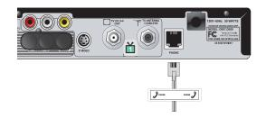
*d.* Connect the remote antenna to the "Remote Antenna" port on the new receiver.
