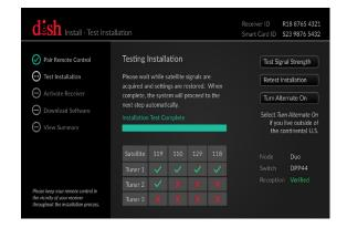
If red "X's" appear in the installation summary, ensure that the "Home Video Network" cable is firmly connected to your Hopper 3 and the wall. Then, use your remote control to highlight "Retest Installation" and press SELECT.
