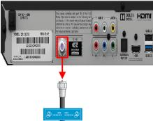
B Locate the cable connected to the "To Hub" port and attach the blue label to it. Then, unscrew this cable from the receiver. Do not unscrew it from the wall.
