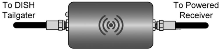
The KING AL1000 Alarm goes in-line between your powered receiver and the DISH Tailgater.
