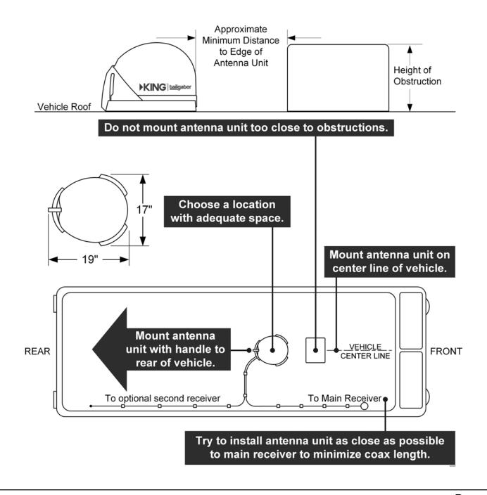
**NOTE:** The installer is responsible for determining the most appropriate fasteners to secure the antenna unit to the roof. Depending on the roof material, fasteners such as lag screws, well nuts, sheet metal screws, toggle bolts and T anchors may be used, and should always be used in combination with a roof compatible sealant.
